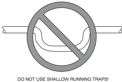
Fig. 18 - Insufficient Condensate Trap
