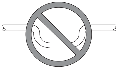
Figure 17 - Siphon de condensat insuffisant
