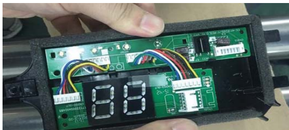
Fig. 23 – Display Board Installed on the Display Board Holder
