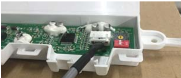
Fig. 25 – Adaptor Board to Display Board Connection
