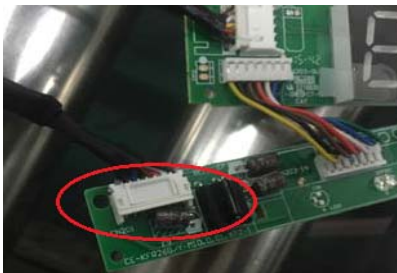
Fig. 19 – CN201 Connection to the Main Control Board
