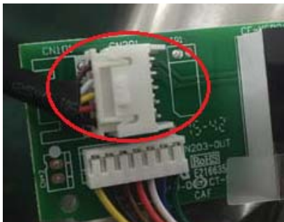
Fig. 20 – CN101 Connection to the Adapter Board
