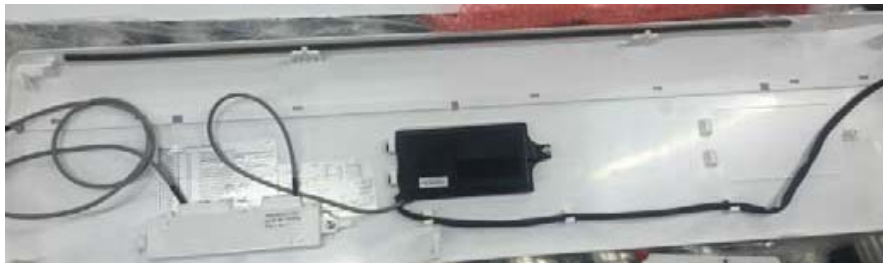
Fig. 28 – Front Panel with New Display Board and Adapter Board
