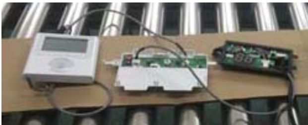
Fig. 18 – Wired Controller, Adapter Board, and Display Board
