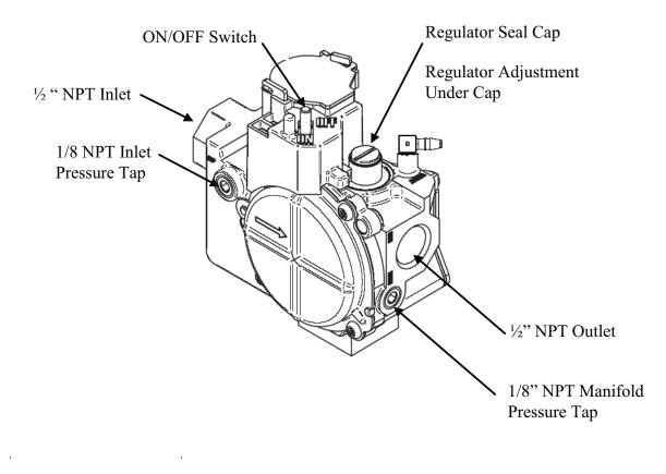
Fig. 1 - Single Stage Gas Valve
