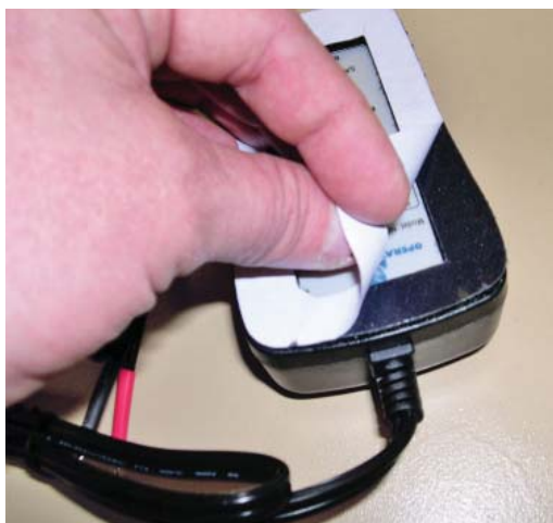
Figure 3.8 — Removal of Adhesive Covering on Hook and Loop for Mounting
