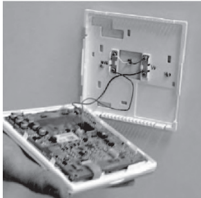
Fig. 10 - Connect Pigtail Wires to Display Module
