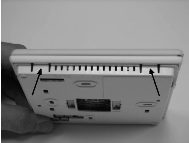
Fig. 5 - Press Tabs to Remove Backplate
