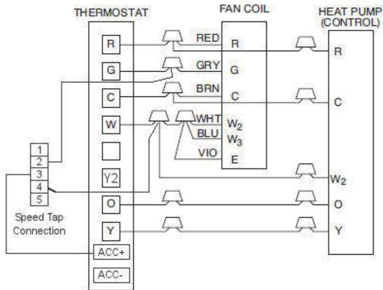
**FX Wiring Layout, Heat Pump Unit
