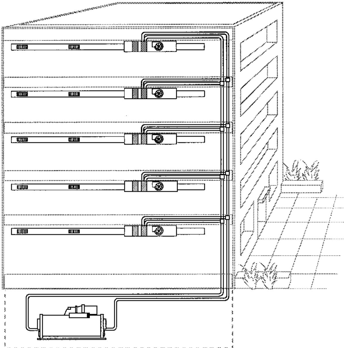
Figure 1-2: Building with Chiller and Air Handlers
