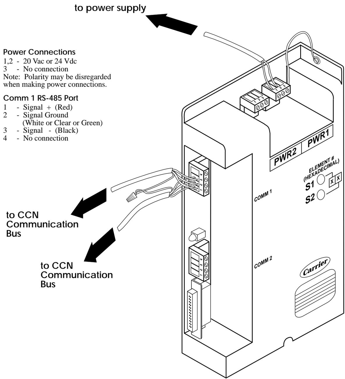
Figure 2-3: Connections for CIO Module Used as a Processor for an Option or a Primary Bus NDS
