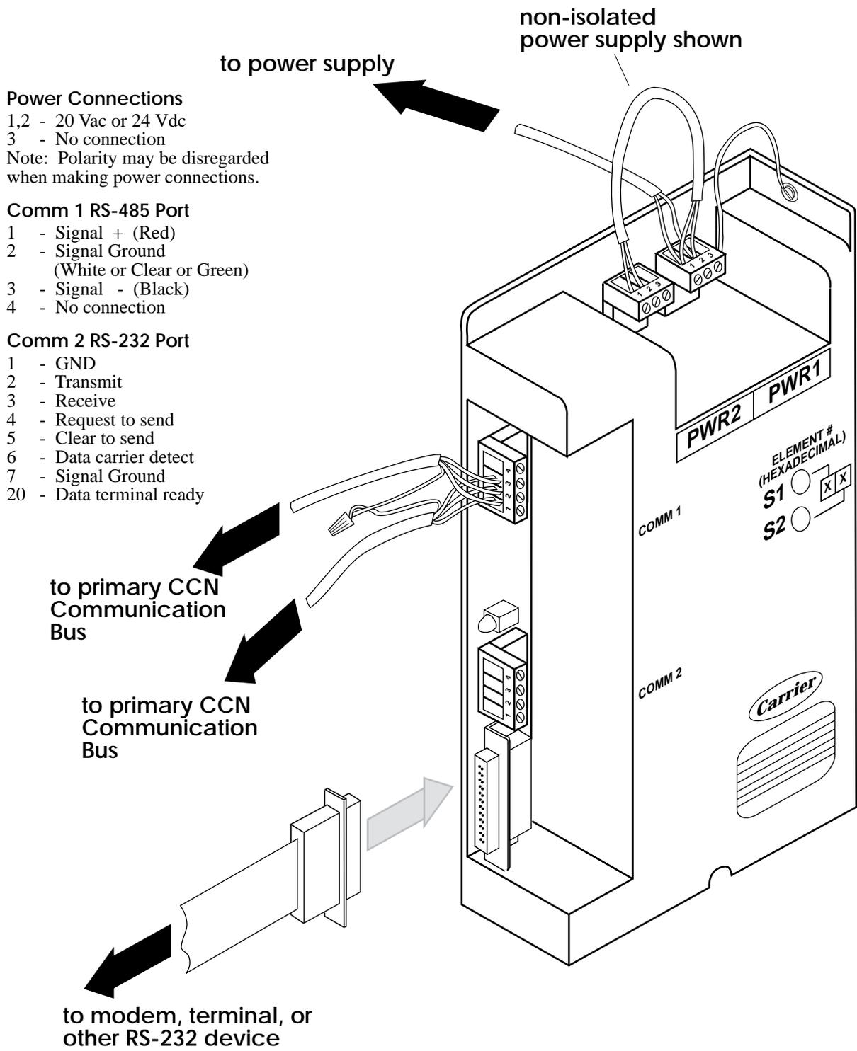
Figure 2-5: Connections for CIO Module Used as an Interface to an RS-232 Device
