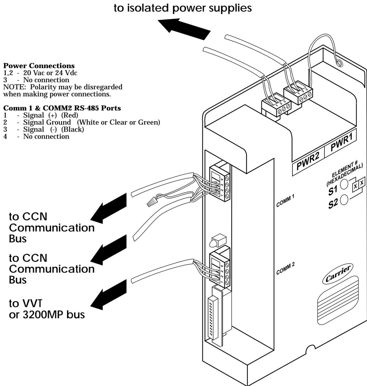
Figure 2-6: Connections for CIO Module Used as an Interface to a Non-CCN Four-Wire Bus
