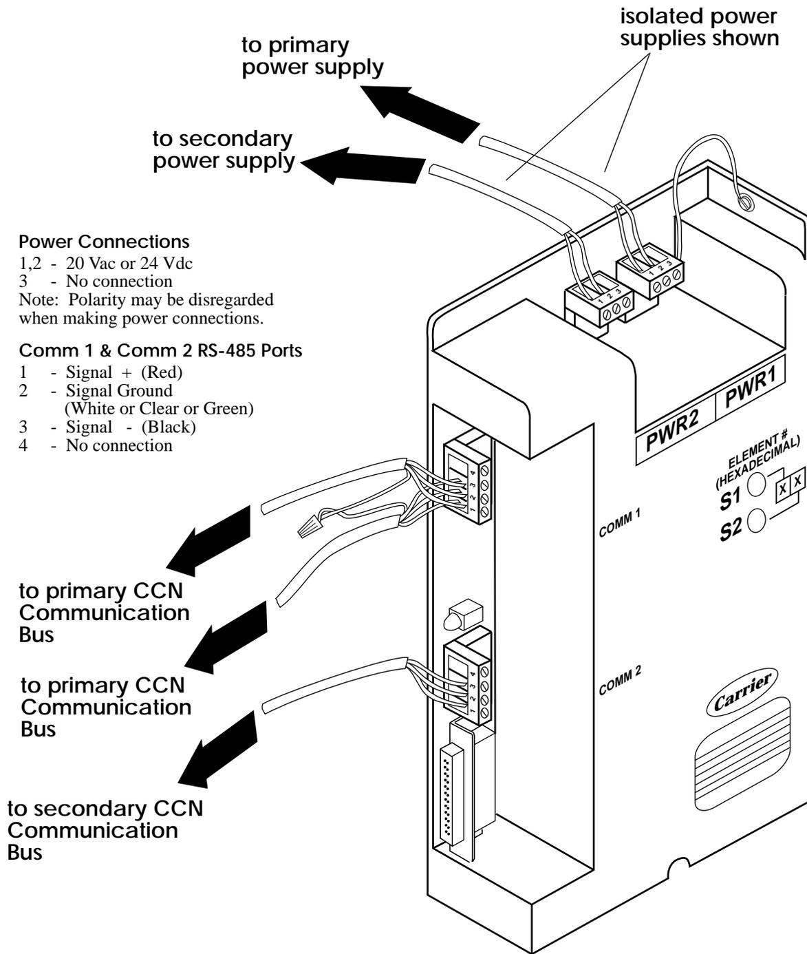
Figure 2-4: Connections for CIO Module Used as a NDS/Bridge
