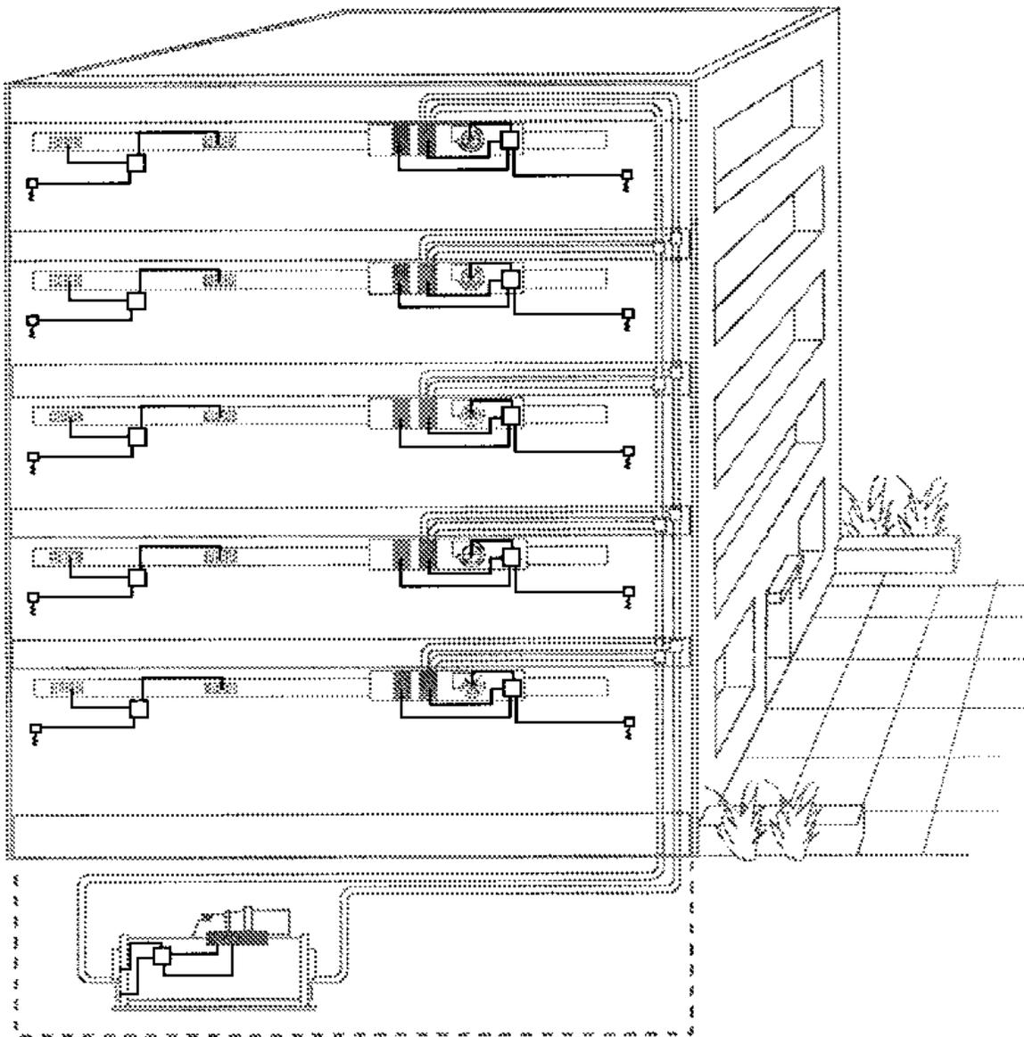
Figure 1-3: Building with Controllers Added to HVAC Equipment
