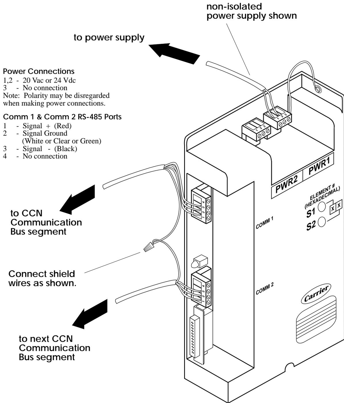
Figure 2-1: Connections for Repeater Used as Bus Extender
