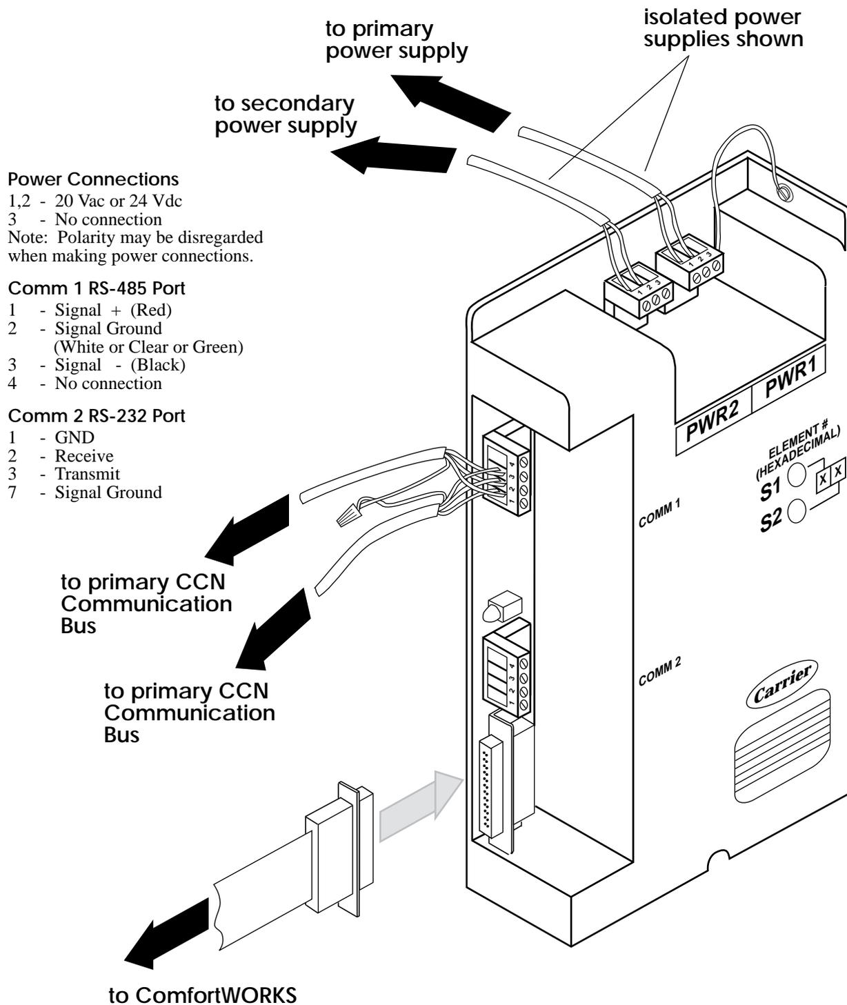
Figure 2-2: Connections for Repeater Used as Protocol Converter
