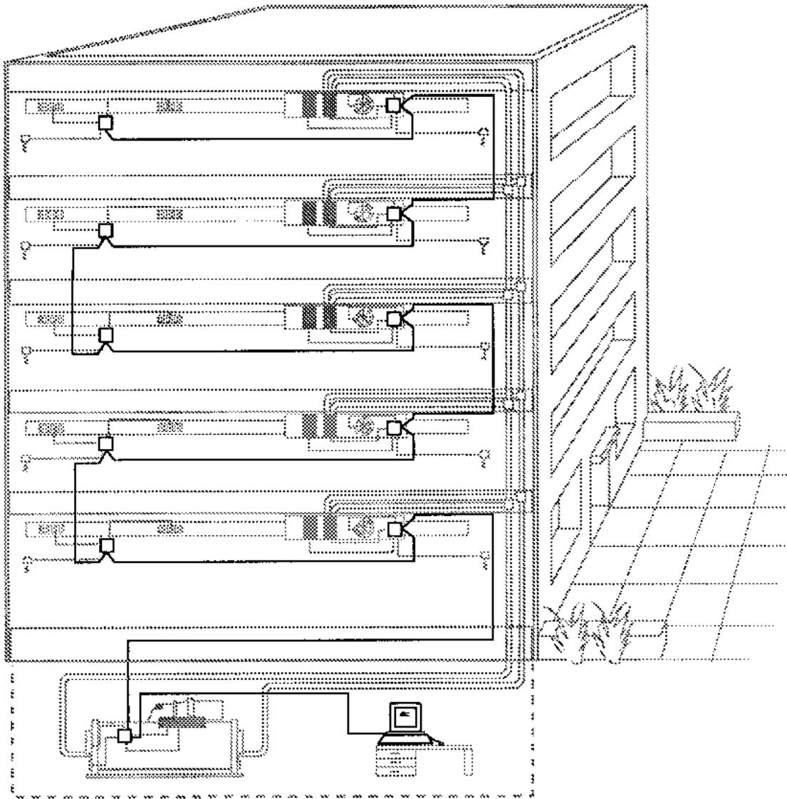
Figure 1-4: Building with CCN Bus and ComfortWORKS Added
