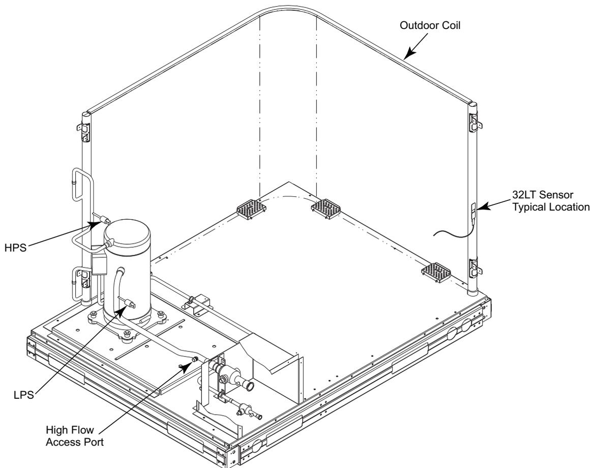
**Fig. 30 - Typical Interior, Single-Circuit Unit (38AUZ\*08 shown)**
