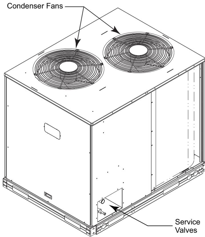
Fig. 31 - Typical Exterior, Two-Circuit Unit (38AUD\*14 shown)
