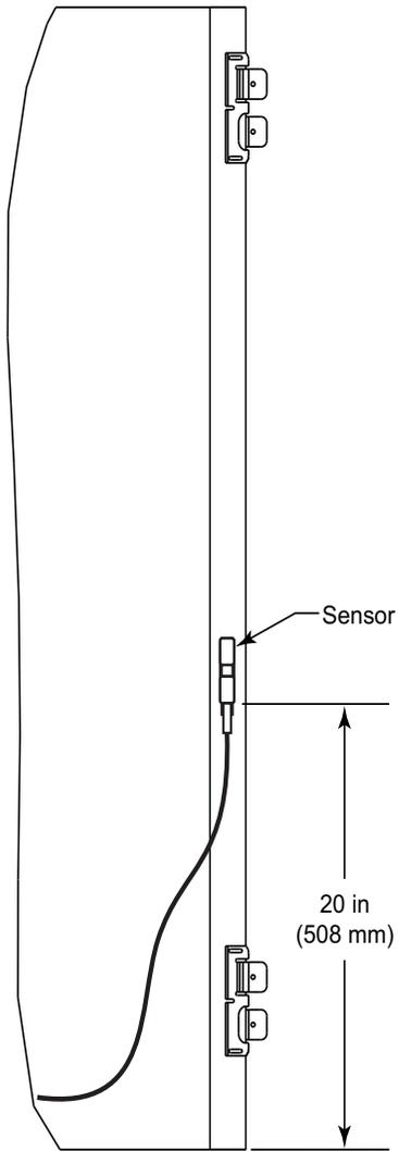
**Fig. 35 - 38AUZ Motormaster Sensor Location
