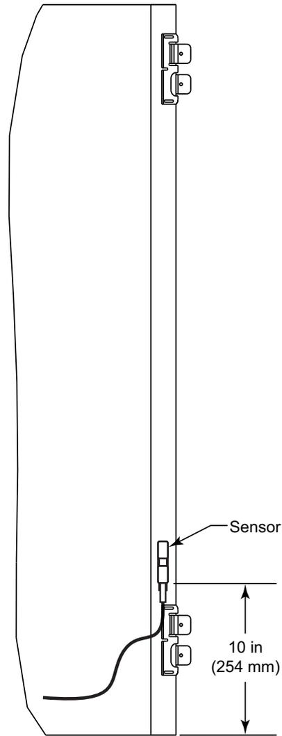
**Fig. 36 - 38AUD\*12-14 Motormaster Sensor Location
