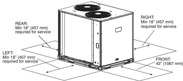
**Fig. 4 - Service Clearance Dimensional Drawing**
