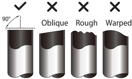
**Fig. 11 — Pipe Cutting**
