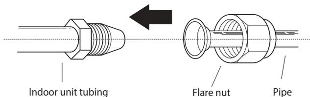
**Fig. 16 — Align the center of the two pipes**
