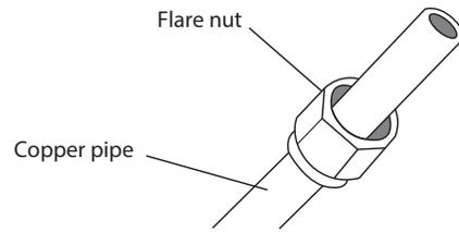
**Fig. 13 — Copper pipe and flare nut**
