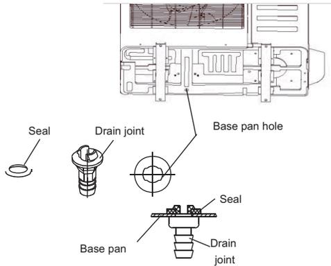
**Fig. 10 — Drain Joint**
