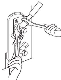
**Fig. 17 — Torque wrench with backup wrench**
