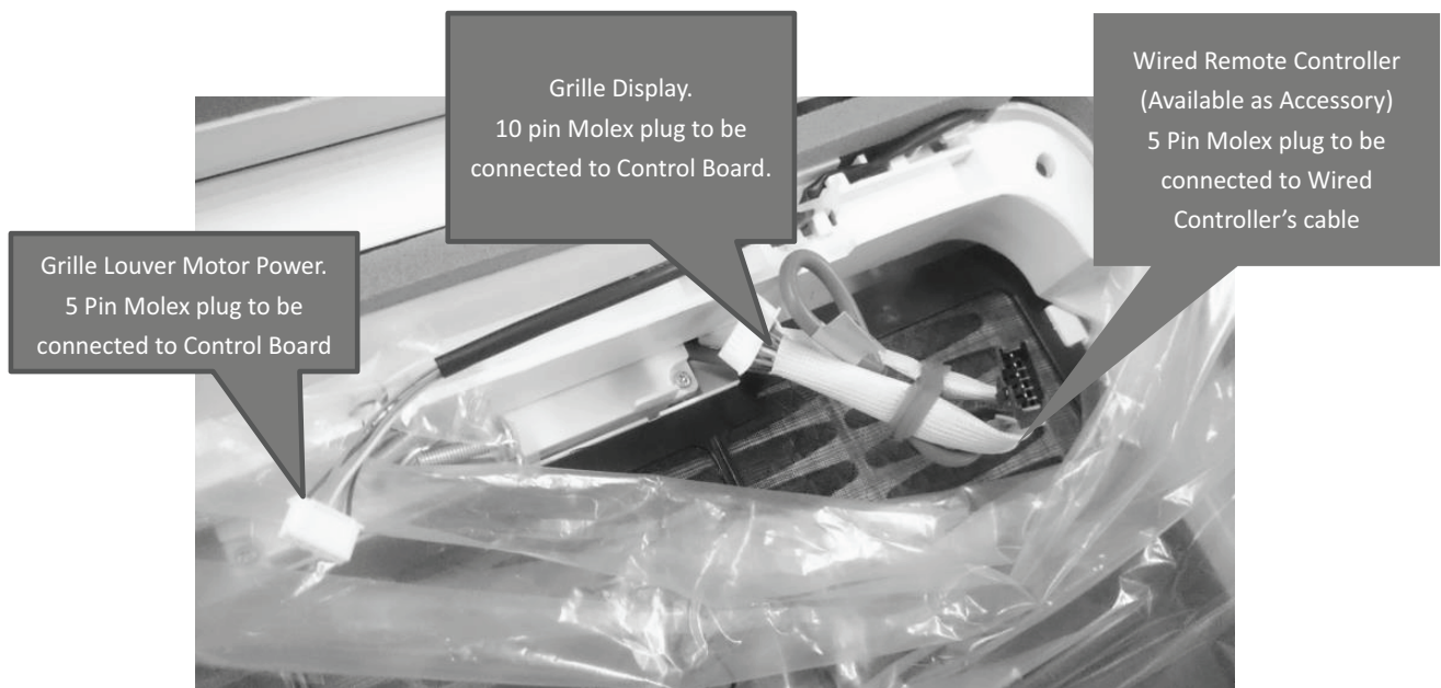
Fig. 29 – Panel Cassette Connections
